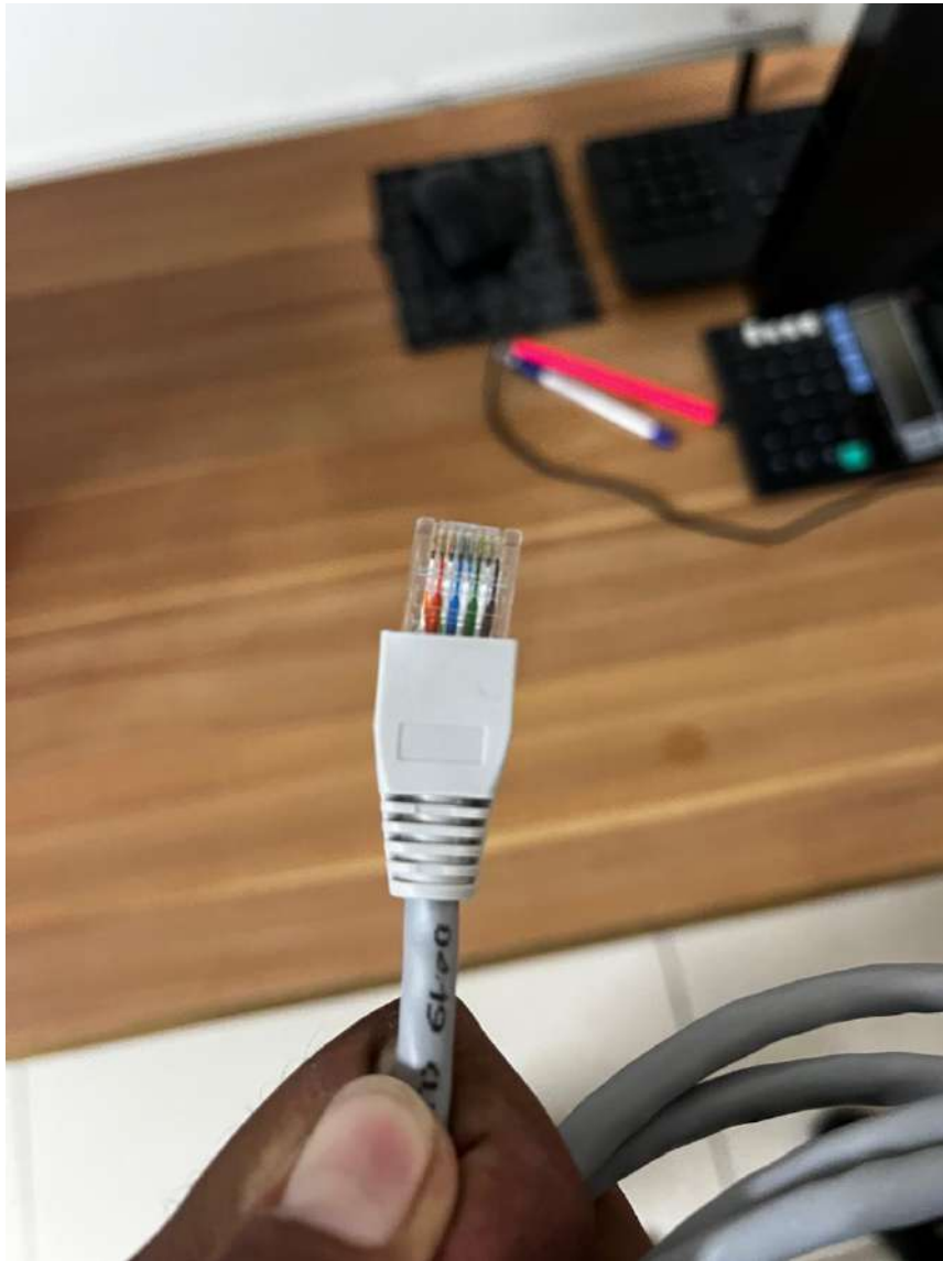
Cat 6 Cable ( Figure 5 )
